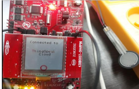
Figure 6: Hardware implementation of proposed system (CC3200, LCD Booster Pack, Pressure sensor).
