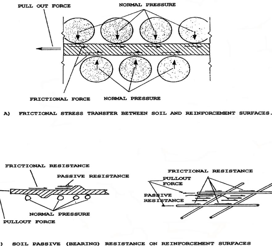
**Figure 2.1** Stress transfer mechanisms for soil reinforcement.(source: FHWA-00-043)
