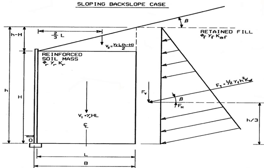
**Note:** For relatively thick facing elements (e.g., segmental concrete facing blocks) it may be desirable to include the facing dimensions and weight in sliding and overturning calculations (i.e. use "B" in lieu of "L").
