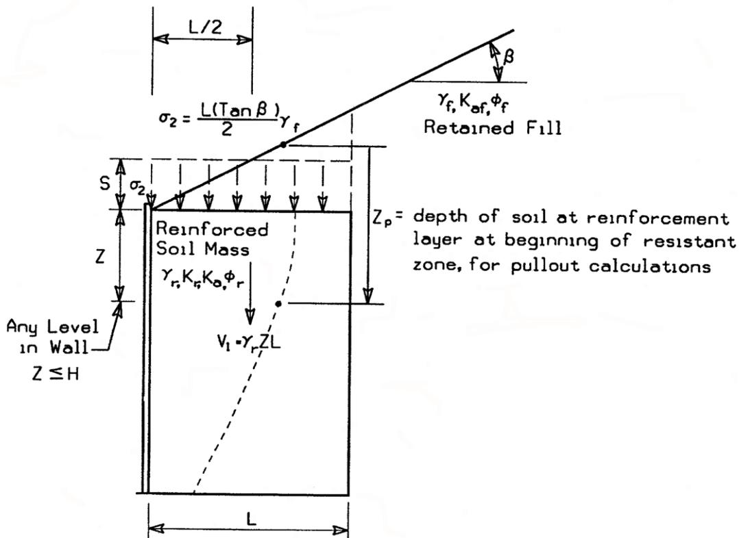
**Figure 8. Calculation of vertical stress for sloping backslope conditions.**
