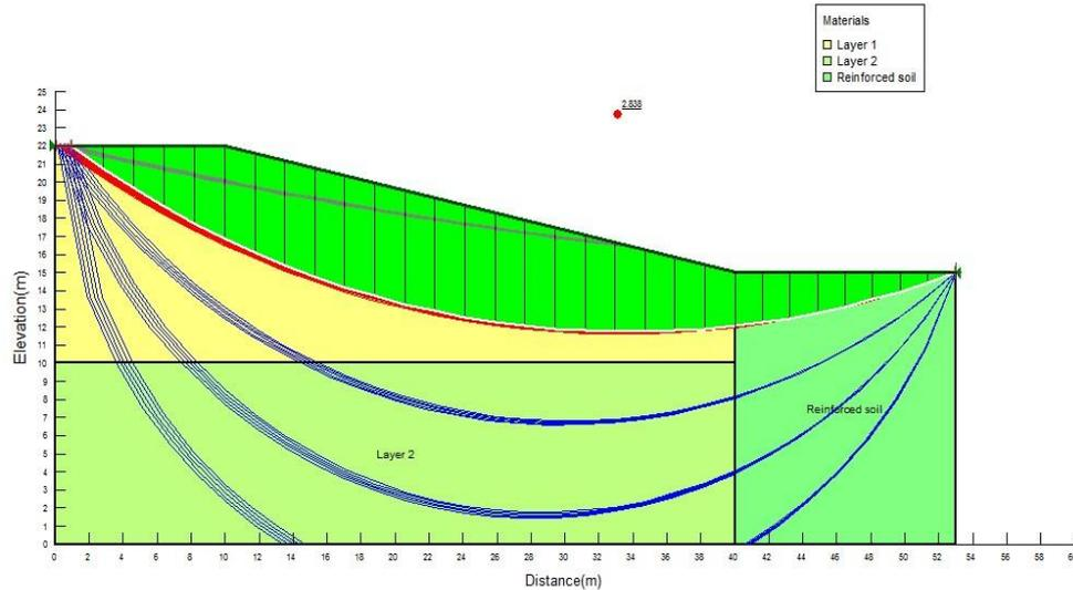
Figure 4.4 Slip circles of the slope
