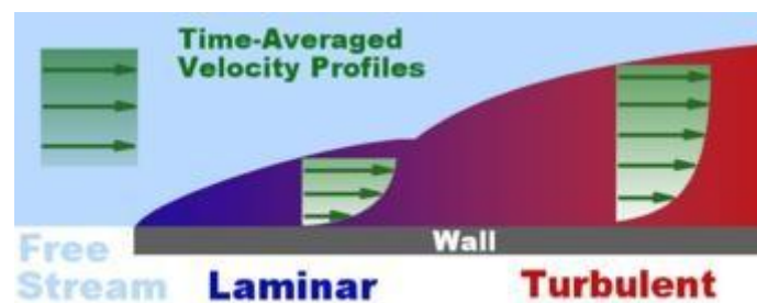
Fig.2. Boundary layer development and transition along a surface
