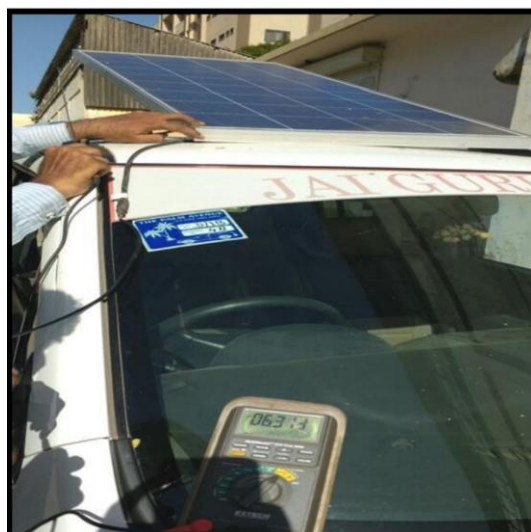
Fig 3.1]Solar panel placed on roof of the car.
