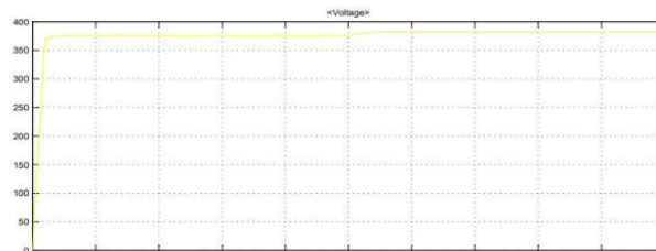
Fig 6 Battery Voltage with BLDC machine
