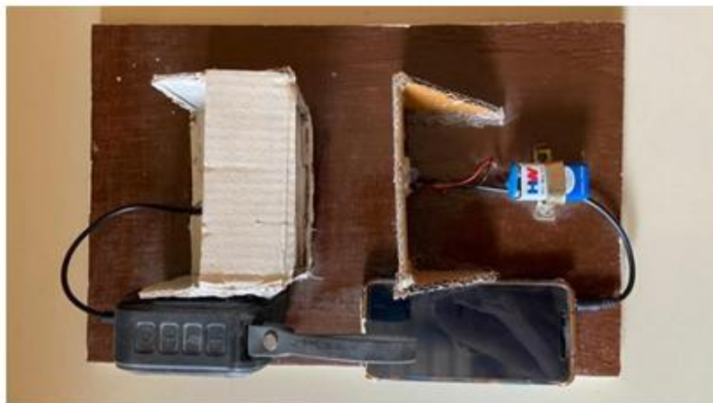
Fig 2. Audio Transmission using Li-Fi
