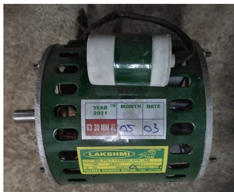
Figure 1: Single phase Motor
