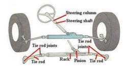
The rack-and-pinion steering gear box has a pinion, connected to the steering column. This pinion runs with a rack that is connected to the steering tie rods. This gives a direct operation.
