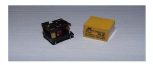
A relay can be defined as a switch. Switches are generally used to close or open the circuit manually. Relay is also a switch that connects or disconnects two circuits. But instead of manual operation a relay is applied with electrical signal, which in turn connects or disconnects another circuit.
