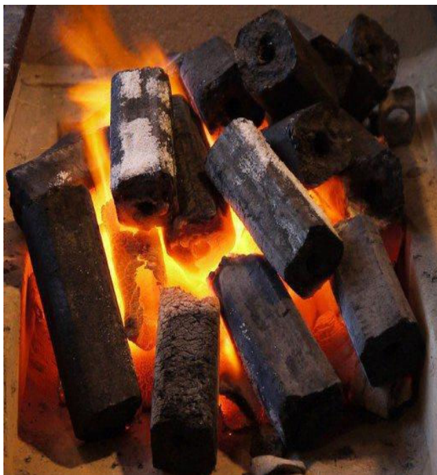
Fig 1: Briquettes from charcoal, wood dust and binder
