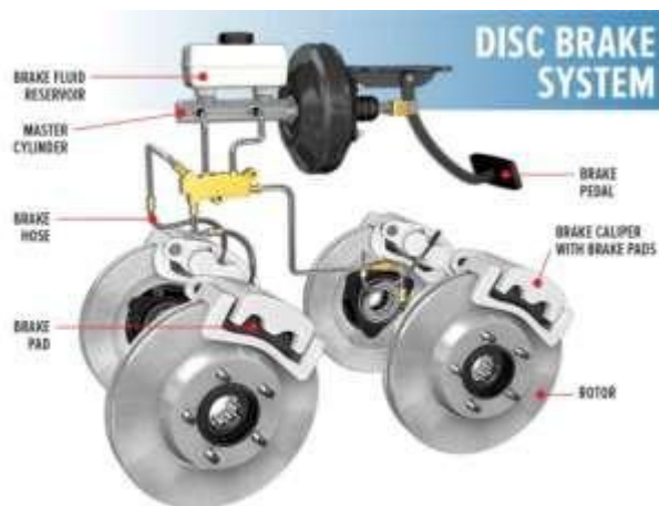
Fig:2 Vehicle disc-braking system
