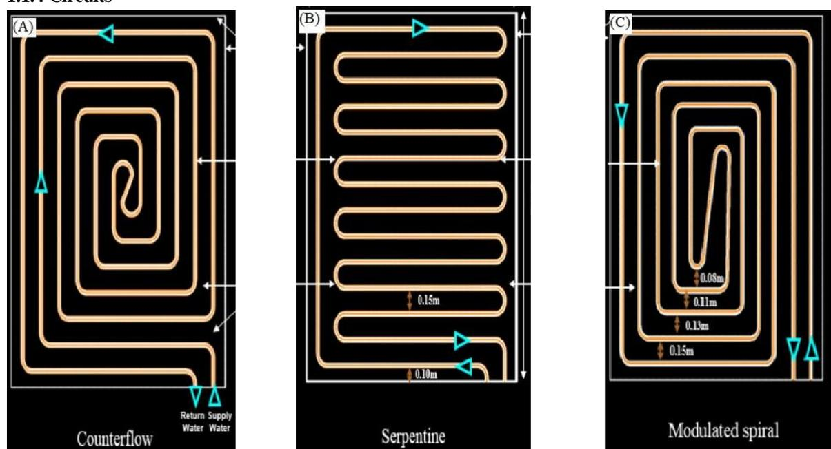
Figure 1 (A) Counterflow (B) Serpentine (C) Modulated spiral
