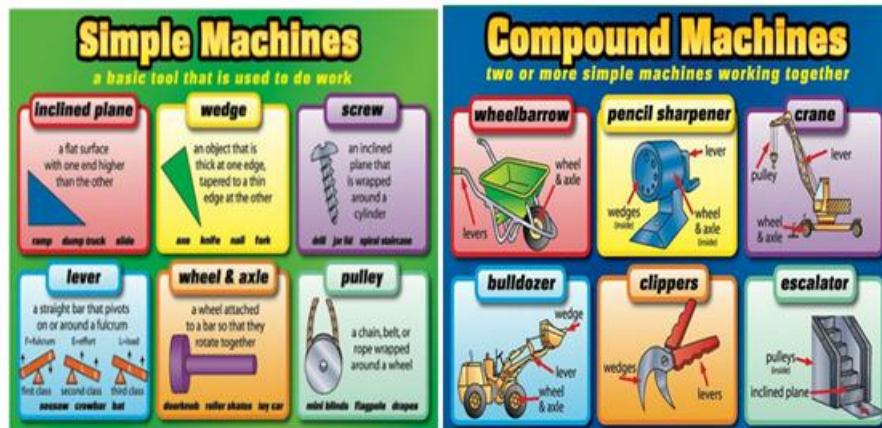
Difference between Simple and Compound Machine
