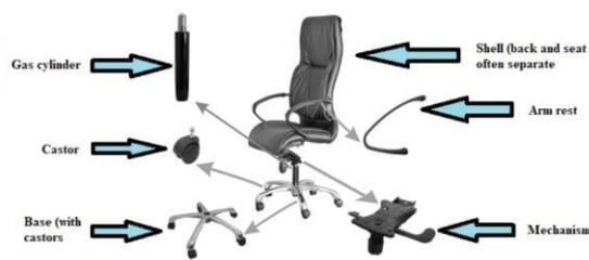
Castor is used in numerous applications, including shopping carts, office chairs, hospital beds and material handling equipment. High capacity heavy-duty casters are used in many industrial applications, such as platform trucks, carts, assemblies, tow lines in plants.
