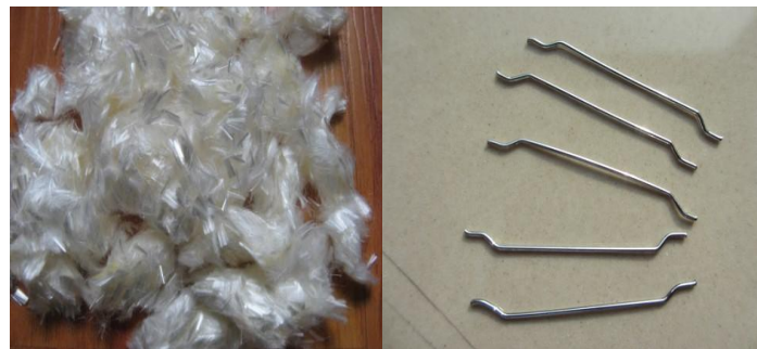
(a).Polypropylene (b)Steel Fig . 2 . Fibres used
