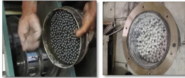
Fig.10. 10 mm stainless steel grinding balls before rinsing and after rinsing with \text{Al}_2\text{O}_3 .
