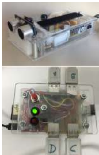
Figure 3: Photography of an air track experiment using the platform. While the mobile unit is on the moving cart, the portable unit stays on the table with four static infrared beacons connected to it.
