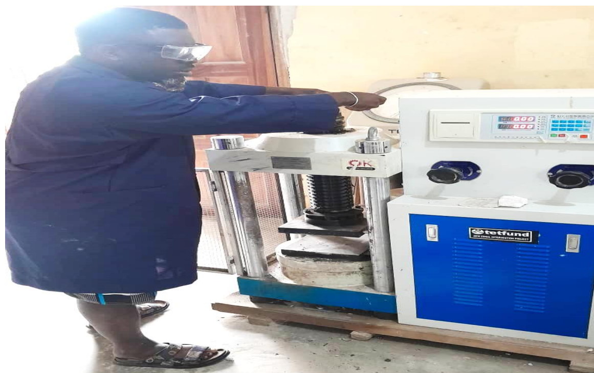
Figure 14: Determination of the Uniaxial compressive strength of rocks from the study area (Source: University of Cross River State Civil engineering laboratory)
