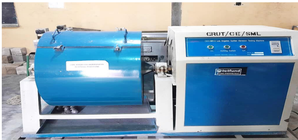
Figure 17: Los Angeles Abrasion test grade B (Source: University of Cross Rivers State Civil engineering lab)
