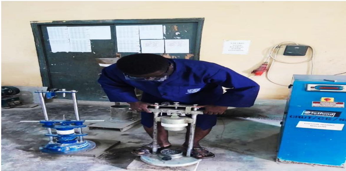
Figure 15: AIV test on representative samples (Source: University of Cross Rives Civil engineering lab)
