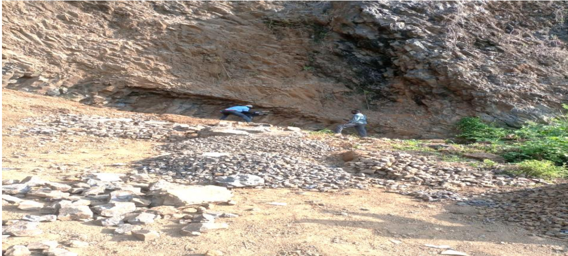
Figure 2: Local basalt quarrying at Ikom (Source; Field work pictures)
