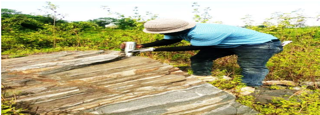
Figure 12: Measurement of in-situ rock strength using L type Schmidt Hammer (Source: Field work)
