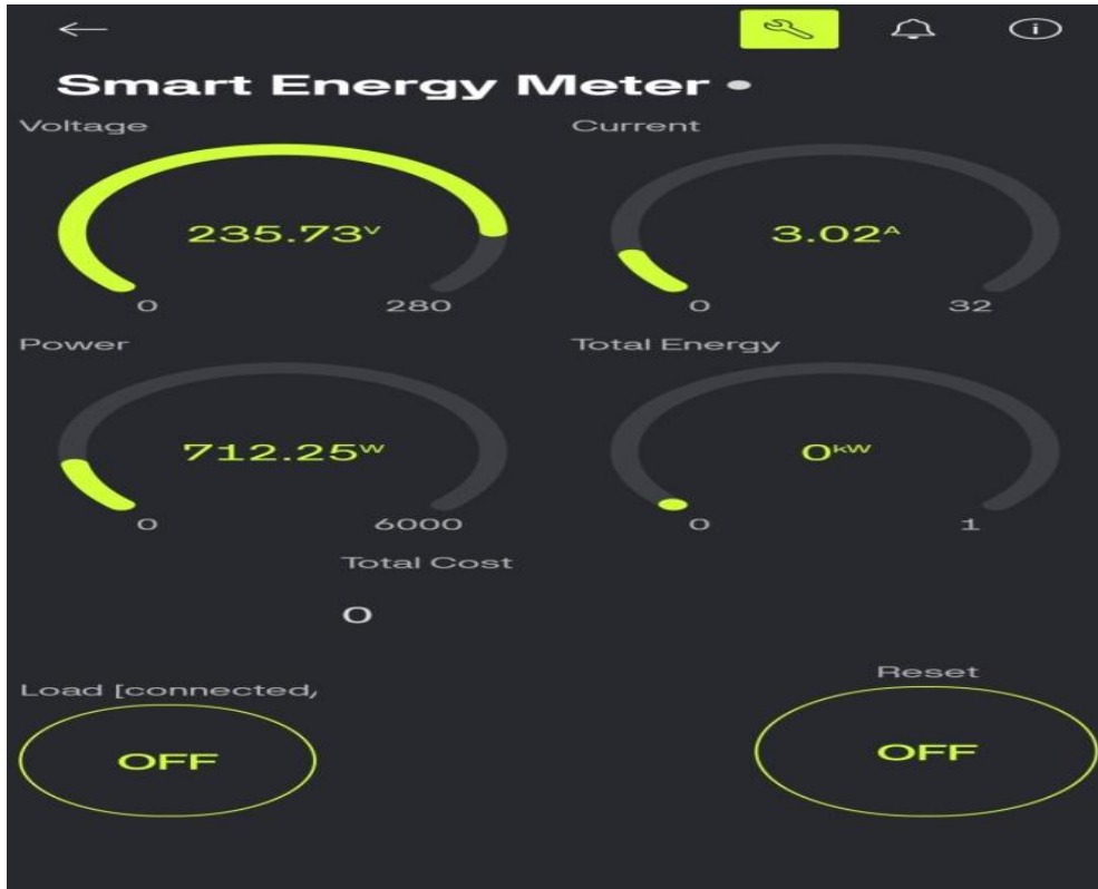
Fig. 4. Blynk IoT dashboard for real-time monitoring and load control with cost reset button
