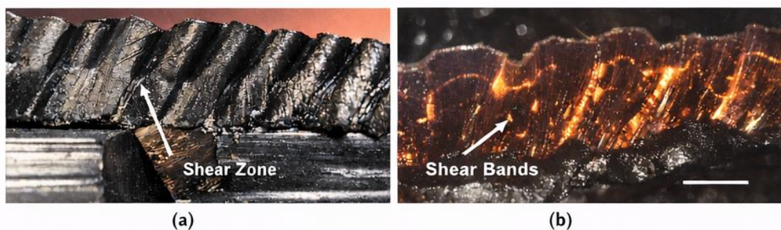
Figure 1. Chip formation in titanium turning: (a) Serrated chip morphology; (b) Adiabatic shear band formation observed under high-speed imaging, Adapted from Li et al. [6] and Sun et al. [1].
