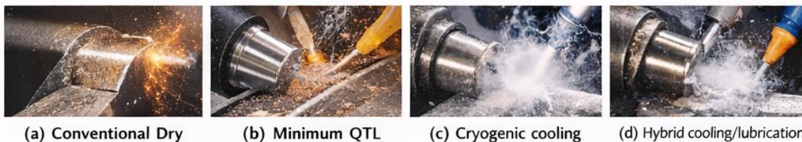
Figure 3. Comparison of cooling and lubrication strategies in titanium machining: (a) Dry cutting; (b) Minimum quantity lubrication (MQL); (c) Cryogenic cooling; (d) Hybrid cooling/lubrication. Adapted from Dhar et al. [9] and Zhang et al. [8].
