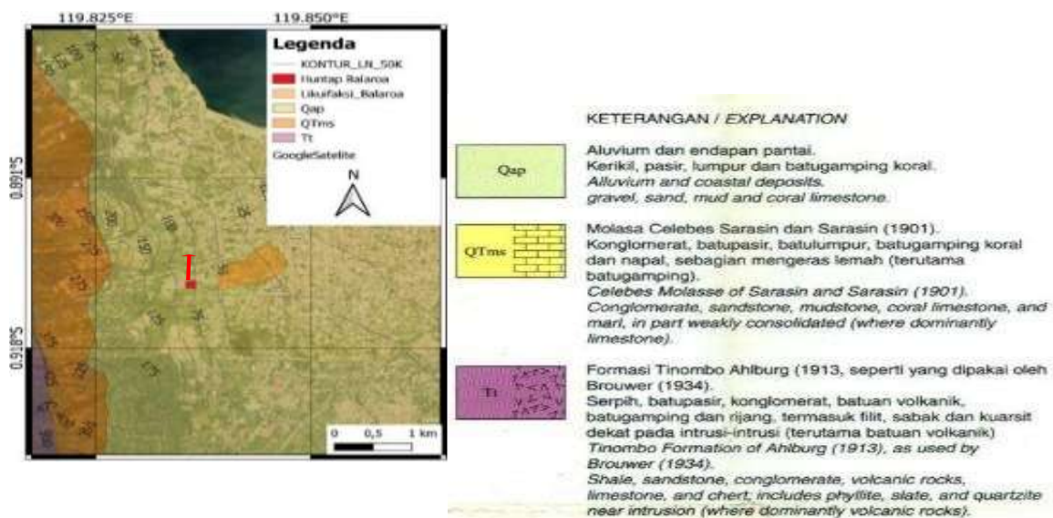
Figure 4: Geology of the Balaroa Liquefaction Area
