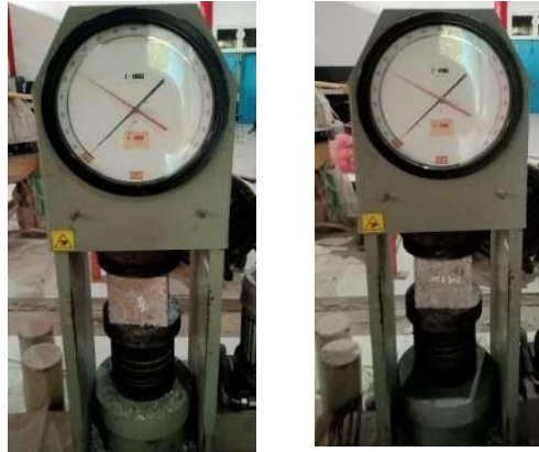
Figure 10 Testing the compressive strength of concrete
