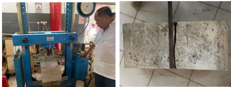
Figure 12 (a) Testing the flexural strength of concrete and (b) Samples of concrete flexural strength test results In testing the flexural strength of concrete, tested as much as
