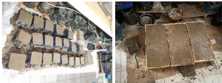
Figure 10 Fabrication of concrete cubes and slabs
