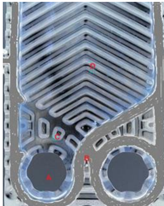
Figure 10. The photograph of a plate of the PHE under investigation. Note the inlet section A, the gasket B, the inlet flow distribution corrugations C and the chevron corrugation D.
