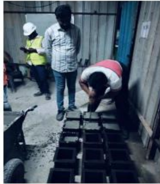
Fig4.2 Casting of fresh SDC mix
