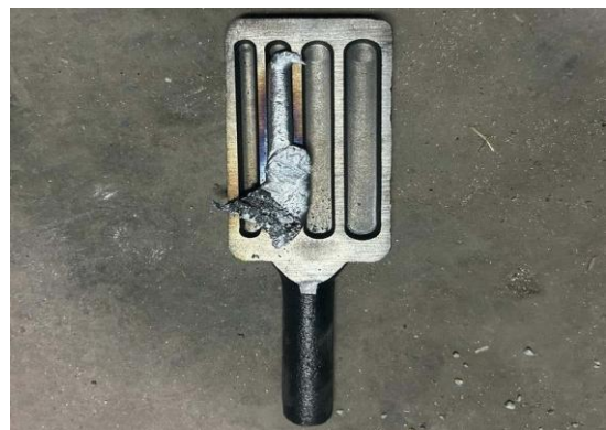
Figure 2 Pouring the molten brazing alloy Figure 3 Obtained Brazing alloy after the mould Solidified
