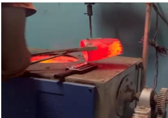
Figure 2 Pouring the molten brazing alloy Figure 3 Obtained Brazing alloy after the mould Solidified
