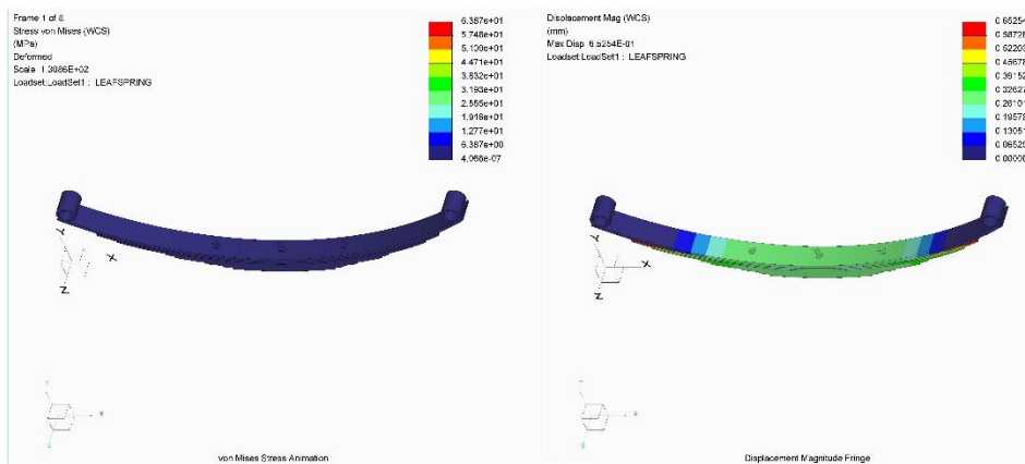
Figure 6: FEA of Leaf Spring made of Carbon Fiber
