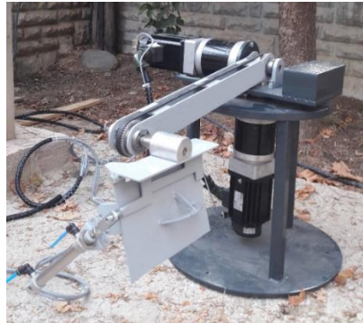
Figure 3: Assembled outer casing of the robotic arm
