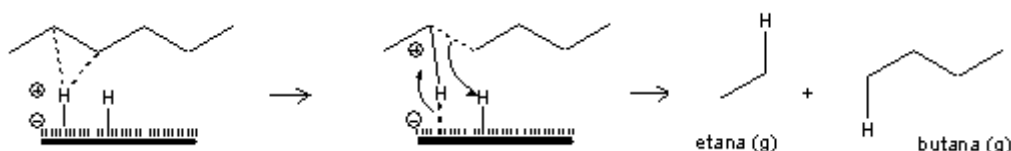
Figure 11. Breaking down hexane compounds into ethane and butane
