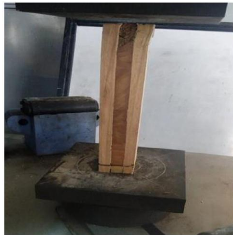
Fig. 2: compression test arrangement using UTM
