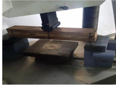
Fig. 1: Shear test arrangement in the Universal testing machine
