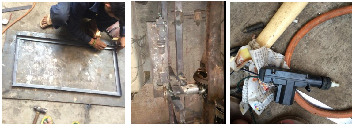
Figure 10 : Frame & Linear Actuator for locking purpose with locking bar
