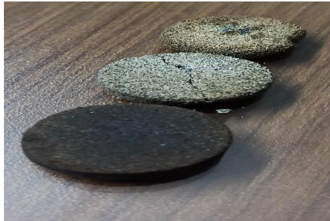
Fig.5: Core slices/discs saturated with brine and aged with crude oil of Upper Assam Oil field.
