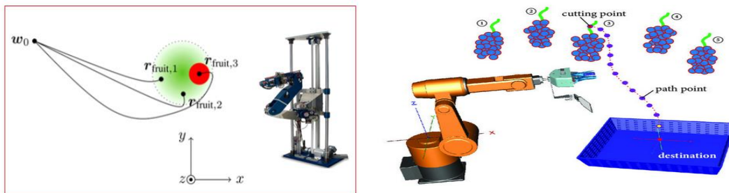
Figure 54 Strategies for fruit harvesting in distributed environments using a heuristic method. for initialising an optimal problem (sweet-pepper) [106] Figure 55 The proposed path-planning method lu et al. [98]
