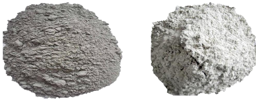
(a) coal ash (b) blast furnace slag Fig.1 Common 3D printed mortar reinforcement materials
