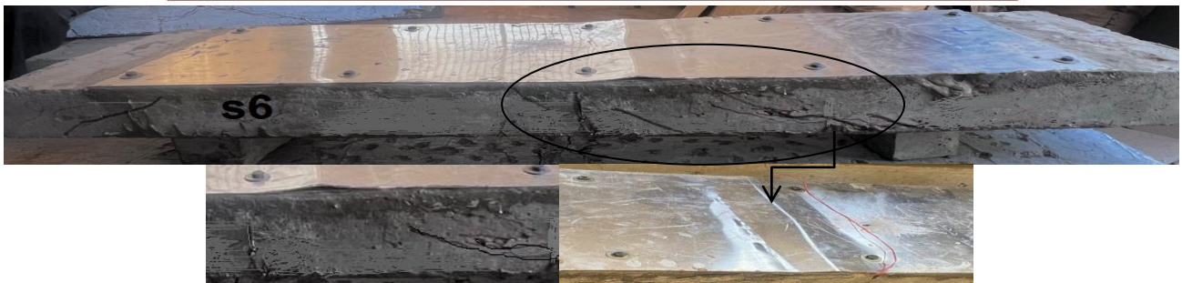
(b): Pattern of cracks of the slab strengthened with aluminum plates at the top and bottom surfaces.
