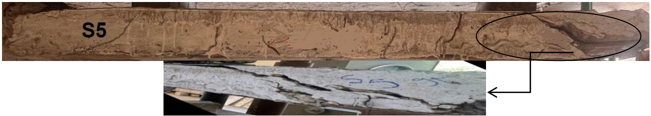
(a): Pattern of cracks of the slab strengthened with steel plates at the top and bottom surfaces.
