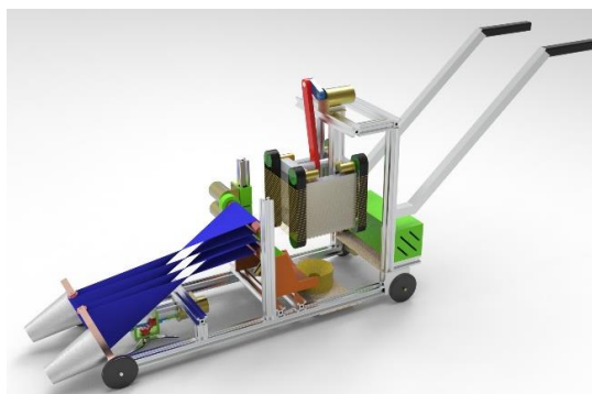
Figure 1: Schematic of the developed chives harvesting and bundling machine
