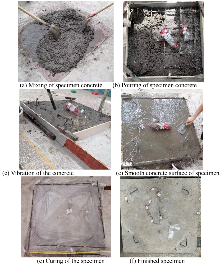
Figure 6: Test specimen production process for the SOAC specimen.
