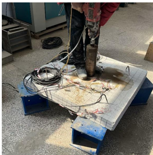
Figure 7: The drilling opening process of the SOAC specimen
