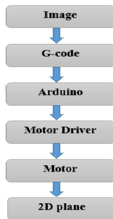
Figure 2: Block Diagram of 2D CNC Plotter
