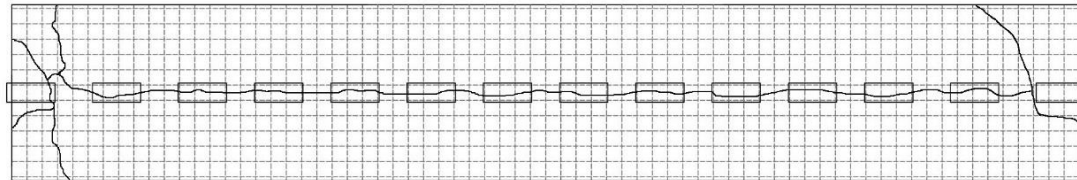
Figure 3.22 Crack distribution on top of concrete slab
