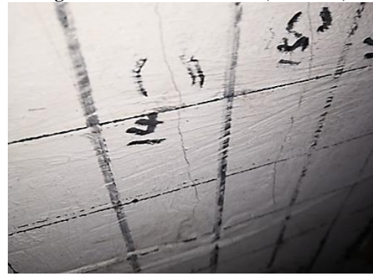
Figure 2.26 Fracture development (Grade 16)
