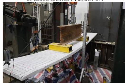
FIG. 2.30 Overall deformation of specimen (grade 17)
