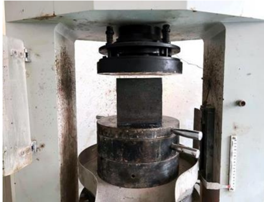
FIG. 2.3 Compressive strength test of concrete
