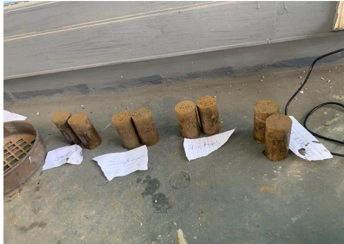
Plate 2: Modified Soil Samples Preparation for UCS Test
