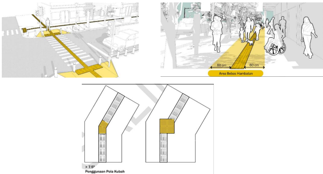
Figure 6: Guide Path according to the Technical Planning Guidelines for Pedestrian Facilities Source: Technical Planning of Pedestrian Facilities of the Ministry of PUPR. 2023
