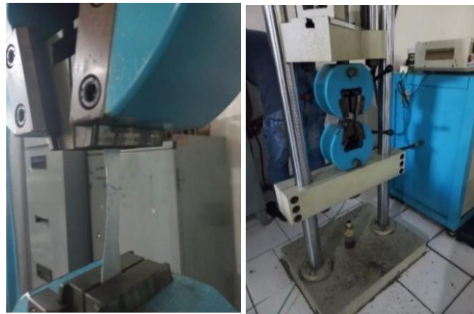
Figure 6: Light Weight Steel Specimen Tension Strength Testing
