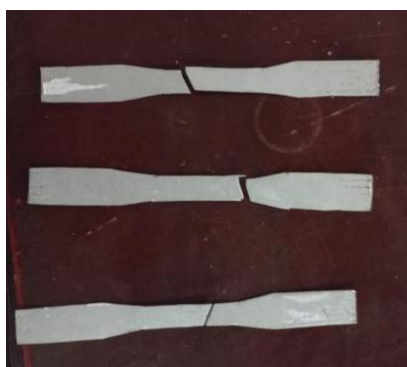
Figure 8: Failure Mode of Specimens
