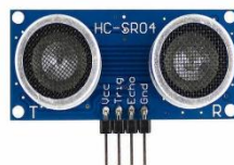
Fig 3. Hardware structure of Ultrasonic sensor
