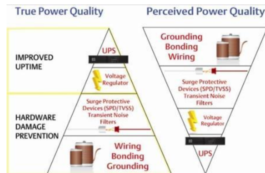
Figure 1 Electrical Power Quality
