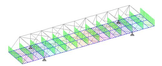
WIND LOAD Wind load / pressure on the structure will be carried out as per IS 875 Part-3 -2015 Wind load for individual Member, coefficient is considered for flat side Member is 1.8.
