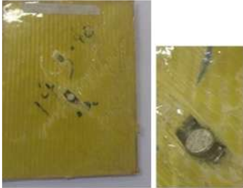
Figure 6 – C1 composite after gunshot test – bullet .38
