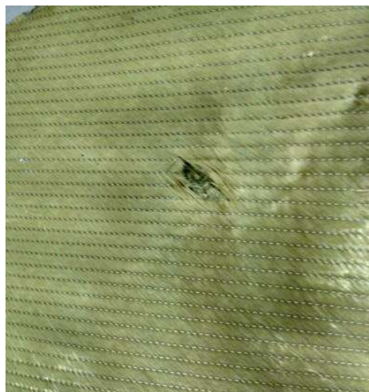
Figure 5 - Bulletproof vest after gunshot test
