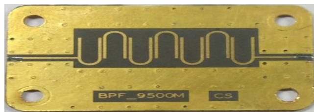
Figure 3: Fabricated microstrip band pass filter
