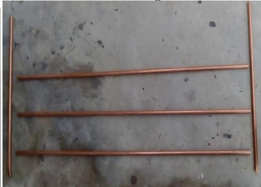
Plate 4 Pipe Assembly of Solar water Heater
