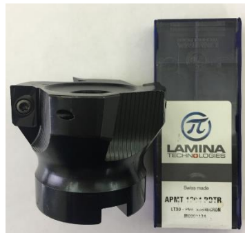
Figure 2. Milling head and carbide inserts used in the experiment
