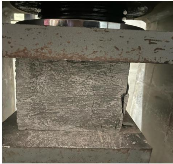
Fig 9 Cube failure under compression
