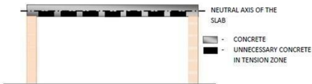
Figure2. Showing unwanted tension concrete
