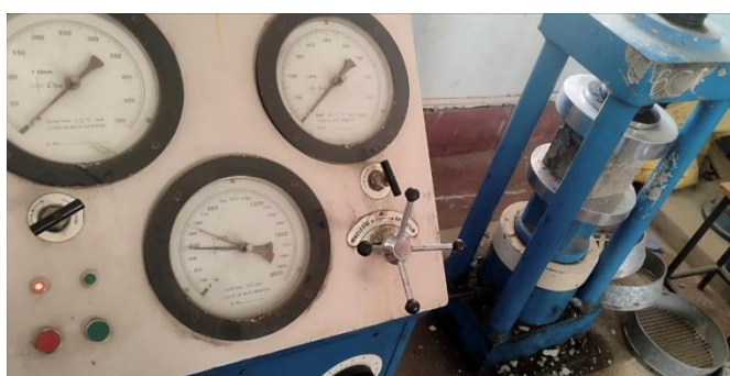
Fig 1: Compressive Strength Testing Machine
